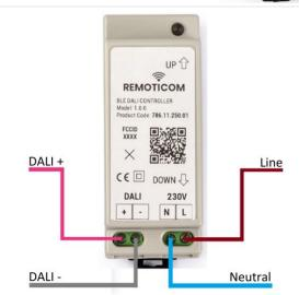
6. After correctly connecting and powering the controller, the LED (marked in red on the side) will turn on shortly and then remain off.
