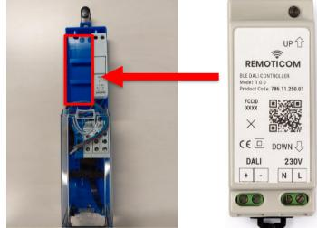
5. Connect the wires to the controller, the connections from left to right are shown in the image to the right:
